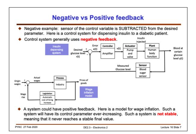
Note that we usually use **negative feedback** in order to control a system. We always subtract the output variable (or some form of feedback value) from the set point, not add.
