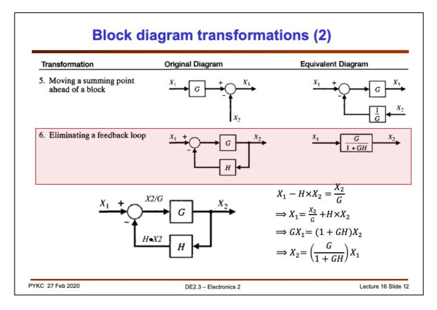
The most important transform is number 6 – transforming a generic feedback loop into a transfer function.
