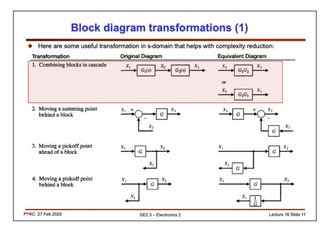
Before we move on, let use consider how to take the block diagram in the Laplace domain and perform some transformations in order to achieve a simplified diagram and to derive the system level transfer function.
