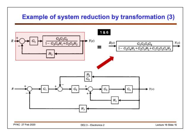
Here we show how the complex block diagram is reduced to the expression shown. Each term in the expression Gx and Hx is a transfer function block in the original diagram.
