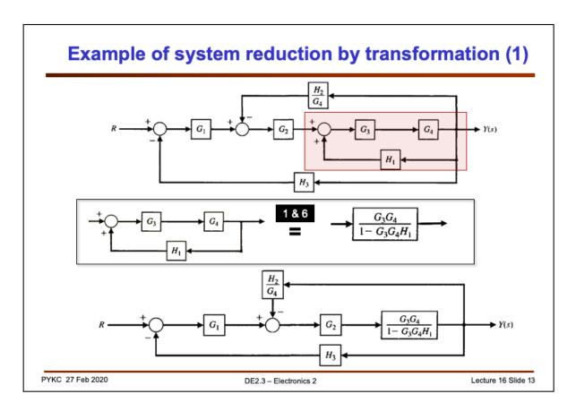
Now let me go through step-by-step how a complex system block diagram can be reduced to a transfer function in the s-domain using an example.
